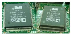
Figure 10: Some pins of the DSP contacted each other.
