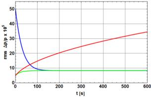
Figure 4: Time development of the relative momentum spread of a beam with  $10^{10}$  antiprotons at 3 GeV interacting with an internal target. The red curve shows the beam heating when cooling is off.
