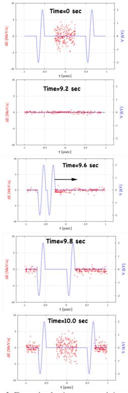
Figure 2: First cycle of antiproton accumulation with a moving barrier. At t = 9.5 s the initially overlapping two barrier pulses are created. One barrier is then moved in the direction as indicated by the arrow. During the barrier motion the beam is compressed to provide new space for injection. The second batch is injected at t = 10 s.
