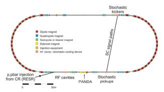
Figure 1: Schematic view of the HESR. The upper straight will accommodate the future electron cooler.
