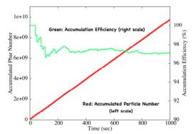
Figure 3: Number of antiprotons during accumulation (red) and accumulation efficiency (green) for the moving barrier scheme.
