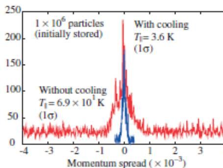
Figure 4 Momentum distributions of a  $^{24}\text{Mg}^+$  ion beam with an intensity of  $1 \times 10^6$  with and without laser cooling [8].
