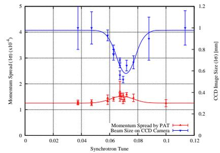
Figure 7 Experimental demonstration of synchro-betatron resonance coupling. Longitudinal momentum spread after laser cooling has a local maximum at  $\nu_s \sim 0.068$  (lower), while the horizontal beam size has a local minimum at the same position (upper).
