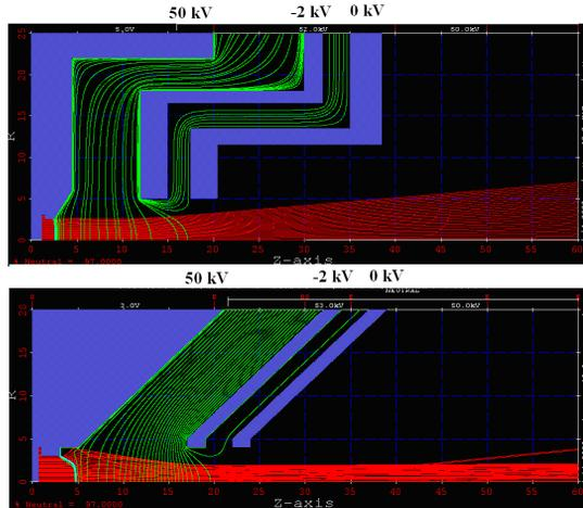
Figure 4: Simulation results of different electrodes.
