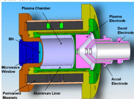
Figure 1: A cut away view of the ion source.
