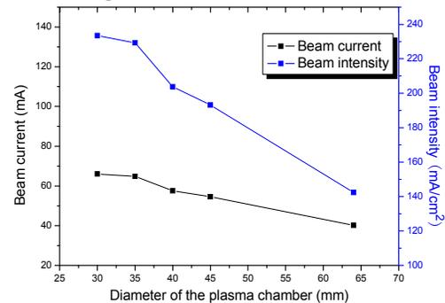
Figure 2: The dependence of beam current and beam intensity on the plasma chamber diameter.
