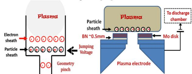
Figure 3: The double layer sheaths caused by geometry pinch (left) and the schematic plot for the pre-accelerator structure (right).
