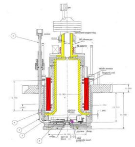
Figure 1: Upgraded design of the Advanced RF Saddle antenna SPS with RF plasma gun for pulsed RF discharge triggering (yellow-ceramic AlN; red-magnetic coil; orange-saddle antenna; magenta-magnetic insert ring).
