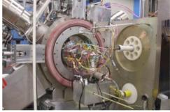
Figure 3: RF SPS saddle antenna, magnetic coil, and external Cs source attached to the test stand.
