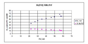
Figure 5: Evolution of the Faraday cup current  $I_{\rm fc}$  and ratio  $I_{\rm fc}/P_{\rm rf}$  as function of  $P_{\rm rf}$  during cesiation. The efficiency of  $I_{\rm fc}$  generation increased with decreased gas flow Q from 20 sccm to 17.2 sccm.
