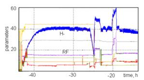
Figure 4: Evolution of H- beam intensity with variation of RF power and magnetic field.
