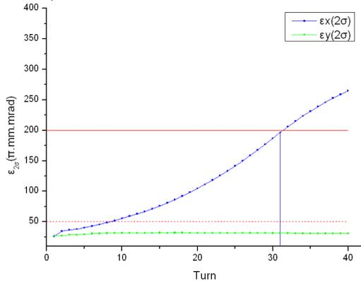
Figure 5: Horizontal emittance growth during injection
