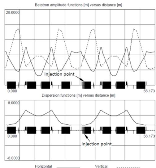
Figure 2: Betatron amplitude and dispersion function of the HITFiL synchrotron ring
