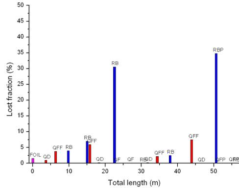
Figure 7: Particles lost position around the ring
