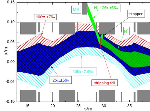
Figure 3: Injecting and coasting beam envelope
