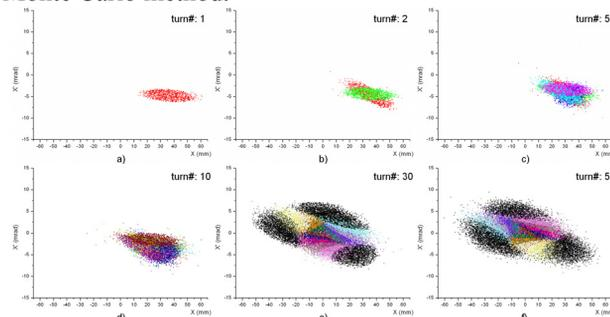
Figure 4: X-X' phase space evolution during injection
