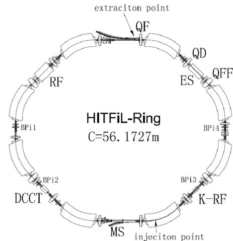
Figure 1: Schematic layout of the HITFiL synchrotron
