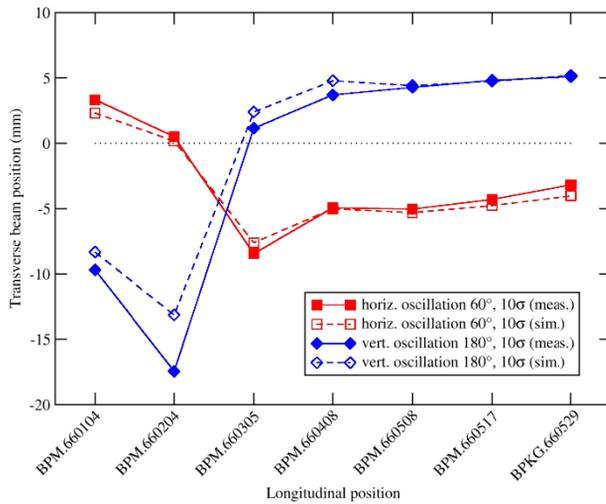
Figure 5: Horizontal and vertical oscillation along the beam line for  $10\sigma$  and phases of  $60^\circ$  and  $180^\circ$ , respectively. The measured and simulated values are shown, which are in good agreement.
