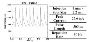
Figure 2: Temporal temperature variation, from the numerical solver with associated parameters [1].
