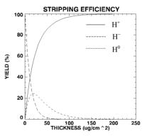
Figure 1: Stripping efficiency of carbon at 180 MeV. Percentage yields of H<sup>+</sup>, H<sup>-</sup> and H<sup>0</sup> are shown.
