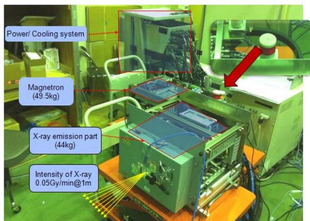
Figure 1: Upgraded X-band 950KeV Linac.
