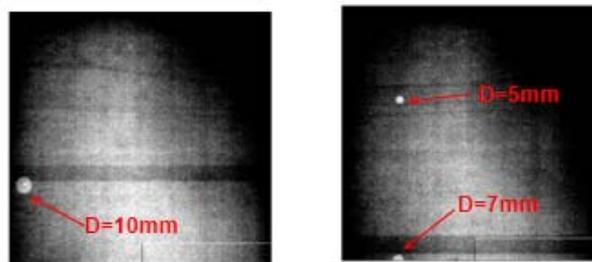
Figure 3: Artificial defects measured by 3.95MeV Linac with scintillation detector for 2s integration time.
