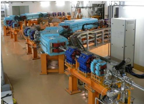
Figure 2: High energy beam transport line (horizontal).
