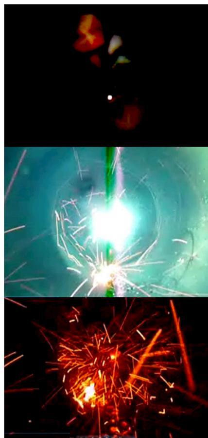
Figure 6: Inconel® RF-contact at 400 A/cm DC corresponding to 75 A/cm at 176 MHz.
