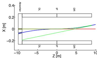
Figure 6: Radiation envelope for the linac-ring design.
