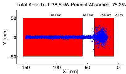
Figure 3: Power distribution on the face of the radiation absorber for the high acceptance layout.
