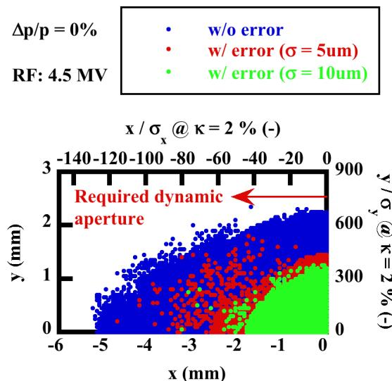
Figure 4: Dynamic aperture for on-momentum particles with Sx-alignment error at injection point.
