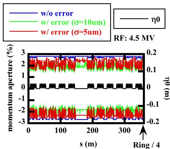
Figure 5: Momentum aperture with Sx-alignment error.
