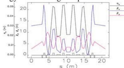
Figure 2: Optical functions of one period of the FBA lattice.
