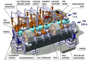
Figure 1: Typical CLIC Two-Beam Module (type 1).
