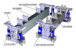
Figure 2: Typical CLIC Two-Beam Module supporting system (type 1).
