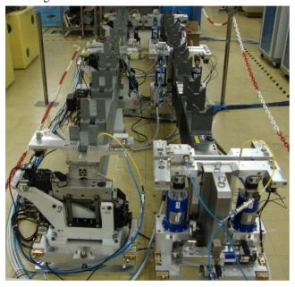
Figure 3: Prototype CLIC Two-Beam Module supporting system (2 test modules type 0).
