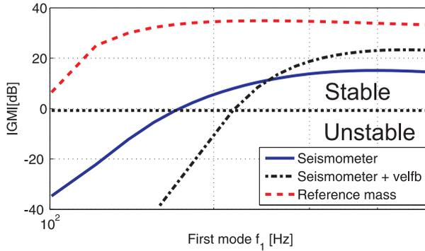
Figure 3: Stability margins for a vibration isolation system with a seismometer, a seismometer with velocity feedback and a reference mass, all with a fixed gain, in function of the first mode of the system.
