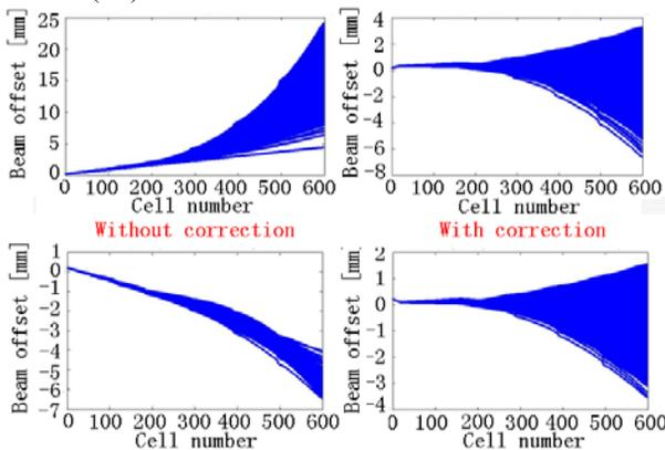
Figure 3: Beam offset distribution of one 0.85A (gun exit)/ $2.7\mu\text{s}$  beam along the whole linac.
