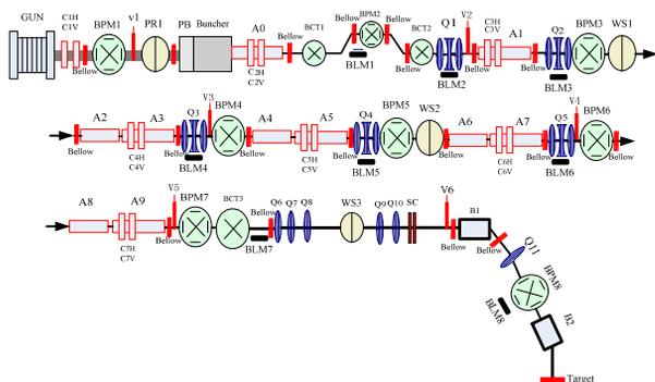
Figure 5: Beam Diagnostic Components.
