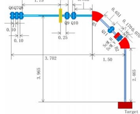
Figure 4: Layout of the transport line.
