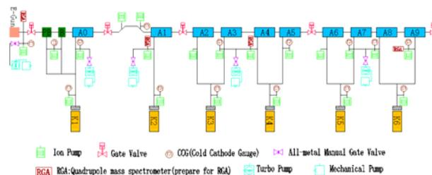
Figure 6: Vacuum system for NSC KIPT Linac.
