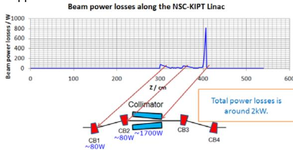
Figure 2: Beam power loss distribution along the linac.
