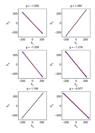
Figure 3: Calibration data from one BPM at CesrTA. Each plot shows the correlation between button signals for 1024 turns of an electron bunch, during resonant excitation in normal mode I. The blue points show the data; the red lines show ellipses fitted to the data. The gradient of the major axis of the ellipse (given as the value g above each plot) gives a component of the calibration matrix B.
