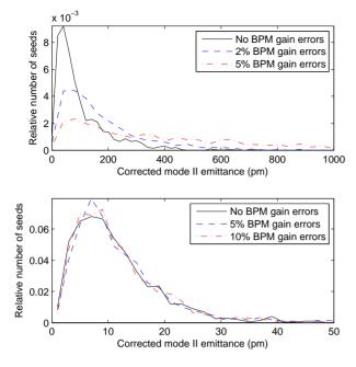
Figure 2: Simulations of emittance correction in CesrTA. Top: distribution of final mode II emittance after orbit and vertical dispersion correction. Bottom: as the top plot, but with correction based on mode II dispersion, rather than vertical dispersion. 1000 seeds of machine error are simulated.
