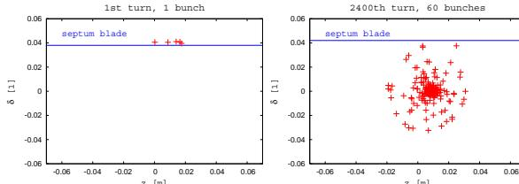
Figure 1: Phase-space snapshots for CLIC-PDR stacking process: first bunchlet on first turn (left), and 60 bunches on turn 2400 (right) [5]. The blue line indicates the location of the septum blade, which changes after the injection turn due to a fast orbit bump.
