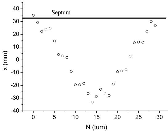
Figure 2: Transverse position of an injected particle at the injection point over 30 successive turns, for an initial momentum deviation  $\Delta p/p_0 = +3\%$  at a dispersion function  $\eta_i = 1\text{ m}$ , an initial betatron-oscillation amplitude  $X_b = 5\text{ mm}$ , a fractional betatron tune  $Q_x = 0.75$ , and synchrotron damping time  $\tau_s = 100\mu\text{s}$  (333 turns).
