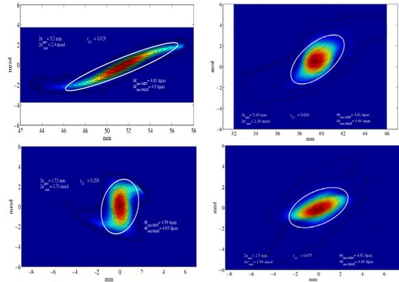
Figure 6: Top: Emittances measured at the Allison-type scanner. Bottom: Emittances determined by linear transformation from the scanner backwards to the quad Q111 entrance. Left: horizontal. Right: vertical. Note that all phase space plots have been drawn with the same scale as Fig. 4.
