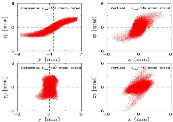
Figure 7: Result of multi-particle tracking simulation with space charge. Top: starting at the emittance scanner. Bottom: tracked backward to Q111 entrance.
