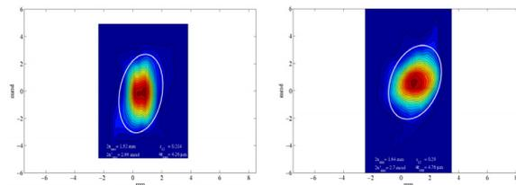
Figure 4: Phase space tomography reconstructed from a series of 1-D profiles measured at WS061. Left: horizontal plane. Right: vertical plane.
