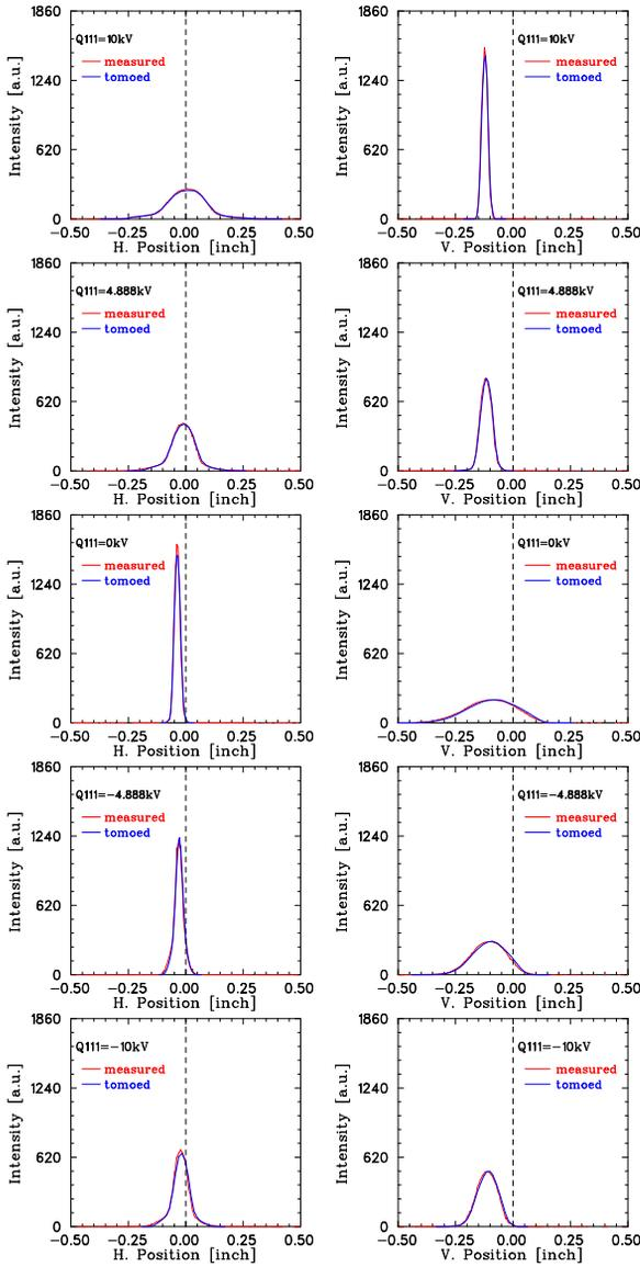
Figure 5: Comparison between the profiles measured and the projections reconstructed from the MENT, at various settings of Q111.
