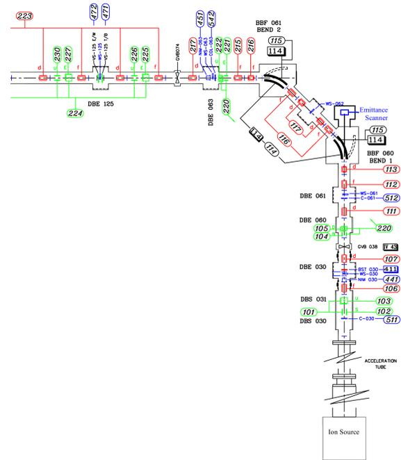
Figure 1: Diagram of TRIUMF 300 keV  $H^-$  injection beamline front end, where the measurements were performed.
