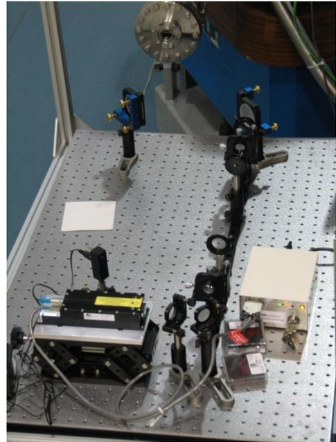
Figure 3: Calibration laser set up with light shaping and steering optics and fast photodiode.
