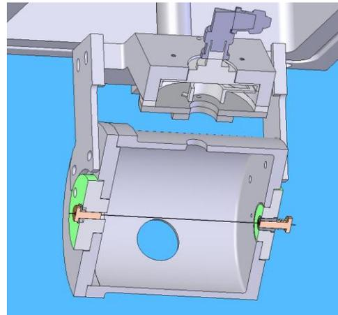
Figure 1: Beam intercepting wire, grounded cylinder and MCP detector assembly on a linear actuator.
