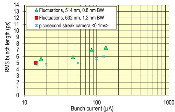
Figure 5: Bunch length measurements in low- $\alpha$  mode ( $\alpha_{\text{nom}}/10$ ) from HU640 radiation,  $V_{RF}=4$  MV.
