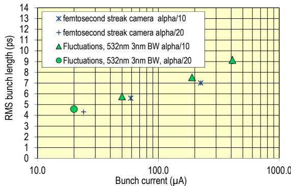
Figure 4: Bunch length measurements in low- $\alpha$  modes from HU640 radiation,  $V_{RF}=3.2$  MV.
