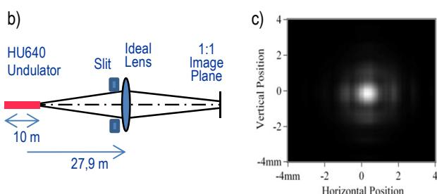
Figure 3: HU640 SRW calculation a) Undulator resonance energy (single-electron flux through pinhole) and experimental energy (multi-electron flux through finite aperture) b) Single-e radiation propagation scheme for coherence evaluation c) Intensity distribution in 1:1 image plane for the single-e radiation at the experimental energy.
