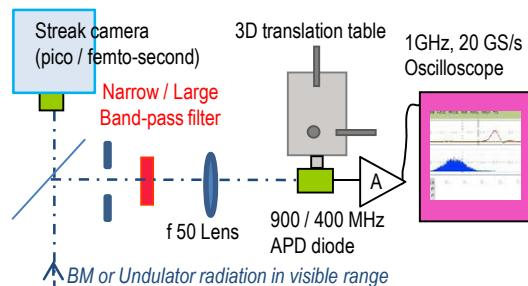
Figure 1: Bunch length measurement setup at SOLEIL.
