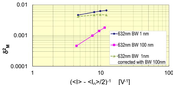
Figure 2: APD parasitic noise evaluation with a large bandwidth filter and fluctuation correction (8 mA 30 ps long bunch, BM).
