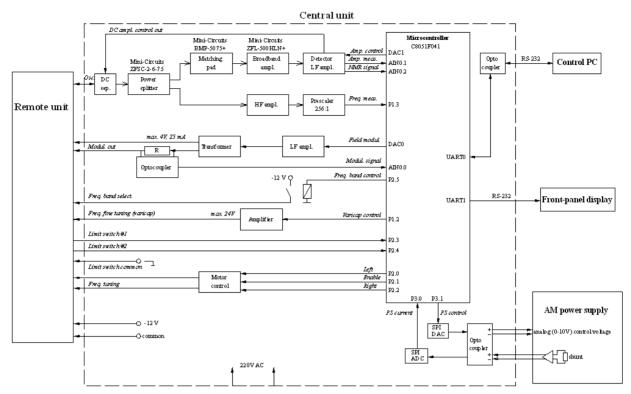
Figure 1: Block diagram of the new central unit with its connections to the rest of the system.
