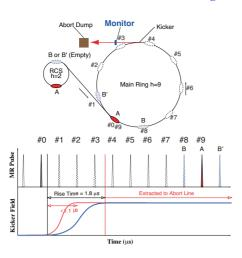
Figure 2: Beam diagnosis by using fast-extracted beam
