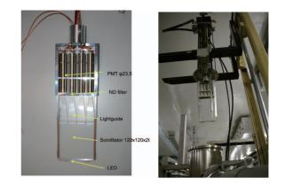
Figure 3: A New beam monitor used for the abort line measurements.
