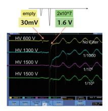
Figure 4: Residual beam in the empty buckets.
