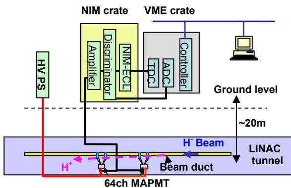
Figure 3: The whole system for beam loss measurements with scintillation fiber hodoscopes.
