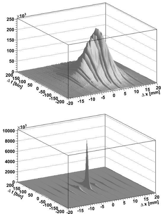
Figure 7: Hit residuals in horizontal position (mm) and TDC bin on H1 with respect to a track connection hits between H0 and H3 (top). Hit residuals on H2 (bottom).
