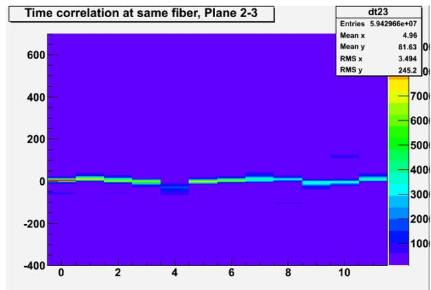
Figure 5: TDC difference (bin) between fiber pairs in H2 and H3 as a function of the fiber number. Fiber 0 is closest to the beam axis. One TDC channel corresponds to 0.2 nsec.
