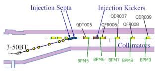
Figure 1: Injection Beam Line of J-PARC MR
