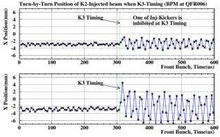
Figure 8: Time-domain horizontal(*x*) position of the K2-injected Front bunch triggered at K3 timing. (Upper): One of inj-kickers is inhibited at K3 timing. (Lower): All inj-kickers are fired at K3 timing.
