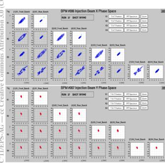
Figure 7: Snapshot of the OPI to show the phase space in physical coordinate for all injected bunches and circulating bunches. Graphs in the gray background are circulating bunches. Upper blue plots are (x, x'). Lower red plots are (y, y'). It is updating in real-time.
