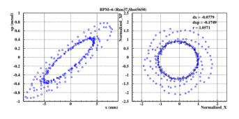
Figure 6: First 230 turns of K1-injected Rear bunch measured by BPM6. (Left): phase space of physical coordinate (x, x'), (Right): normalized coordinate (X, X').
