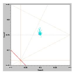
Figure 4: Snapshot of the OPI automatic plotting the tune in the diagram around the operating point (22.40, 20.75).
