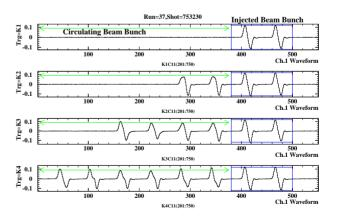
Figure 2: Raw waveform data of BPM ch.1 (from upper to lower, triggered at K1, K2, K3, K4). Couple of bunches surrounded in the blue box are injected beam. The other bunches in the green arrow region are circulating beam.
