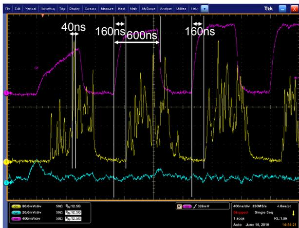
Figure 6: Signals from a gas proportional monitor (blue) and plastic scintillation monitor (yellow) at SDTL13 section, during beam operation with chopped beam. Time scale is extended to 400nsec/div. The beam current signal with a current transformer is also shown (magenta).
