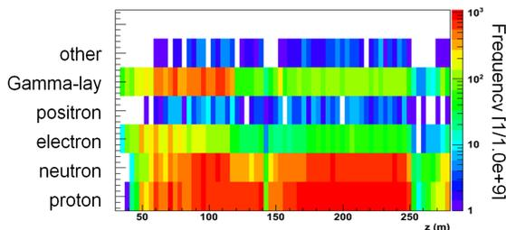
Figure 2: Generated hadrons by the interaction between  $H^0$  and the beam duct.
