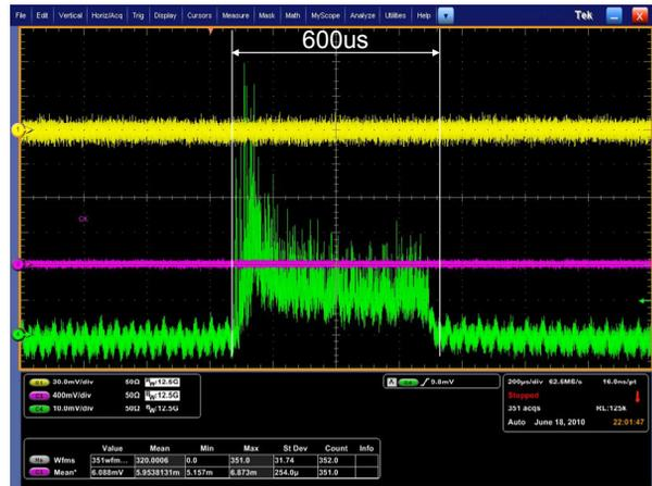
Figure 4: Signals from a gas proportional monitor (green) and a plastic scintillation monitor (magenta) at SDTL13 section, during no beam operation. The beam current signal with a current transformer is also shown (yellow).
