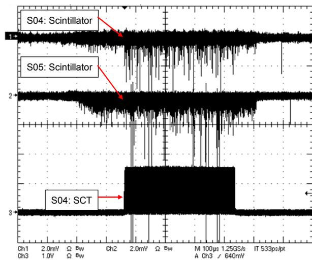
Figure 7: Signals from scintillation monitor installed at the low energy part (SDTL4 & 5). Beam current is also indicated. Signals are mainly detected with the beam current.
