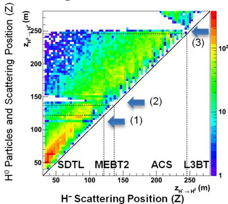
Figure 1: Position and frequency of the scattering between H<sup>0</sup> and beam duct. Negative hydrogen (H<sup>-</sup>) particles are scattered with residual gas and H<sup>0</sup> particles are generated. Generated particles travel to the downstream and scatter with a beam duct.
