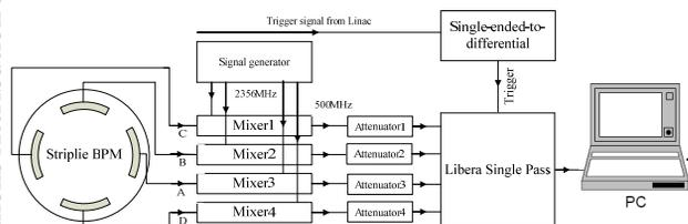
Figure 5: BPM measurement system using Libera Brilliance Single Pass with mixer added.
