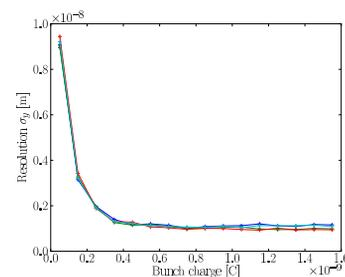
Figure 5: IPBPM simulated vertical resolution as a function of bunch charge.
