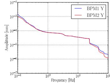
Figure 2: Integrated plot of two IPBPM blocks on the mover system, where the distance between two measurement points is about 20 cm.
