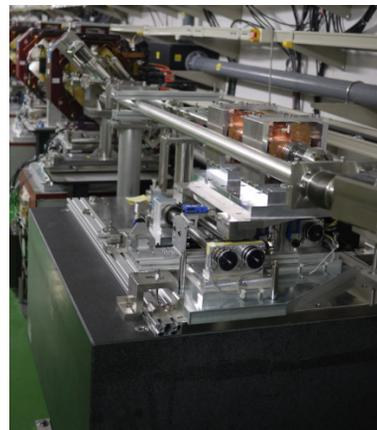
Figure 3: IPBPM system in the ATF2 beam line, located on one of two switchable beamlines, so the IPBPMs installation can be quickly removed without breaking vacuum because the small aperture could introduce wake-fields that distort the bunch shape.
