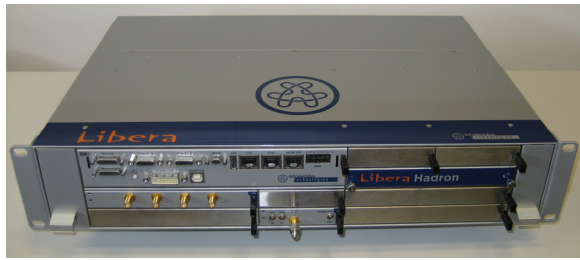
Figure 1: Libera Hadron in a modular uTCA based 19'' 2U rack-mount chassis.
