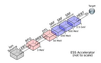
Figure 1: Schematic view of the ESS accelerator.
