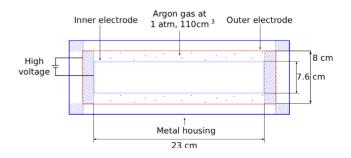
Figure 3: ESS prototype ionization chamber.
