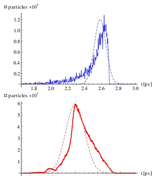
Figure 4: Longitudinal charge profile for bunches with total charge of 0.1 nC (blue) and 3 nC (red). Dashed curves are Gaussian approximations with the same total charge and  $\sigma = 0.1$  ps (blue) and  $\sigma = 0.6$  ps (red).
