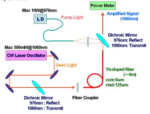
Figure 4: Fiber Amplification Test Setup
