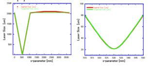
Figure 7: Laser Profile Evolution inside of the Cavity
