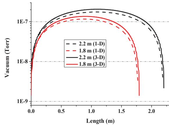
Figure 3: Distribution of the on-axis vacuum pressures along the accelerating column.
