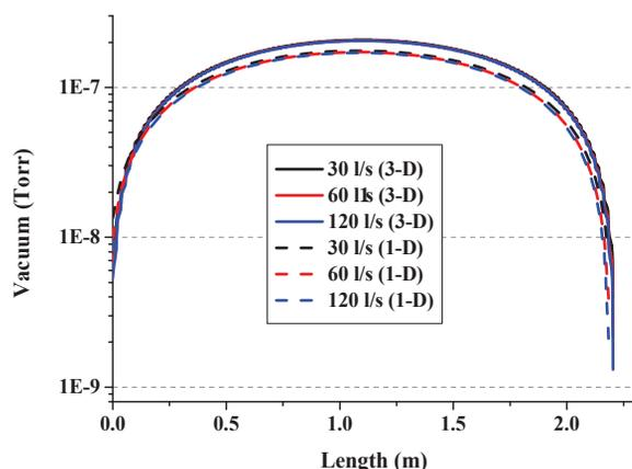
Figure 4: Vacuum pressures with pumping speeds.
