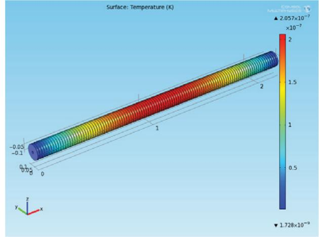
Figure 2: Vacuum simulation model using thermal analogy calculated by COMSOL
