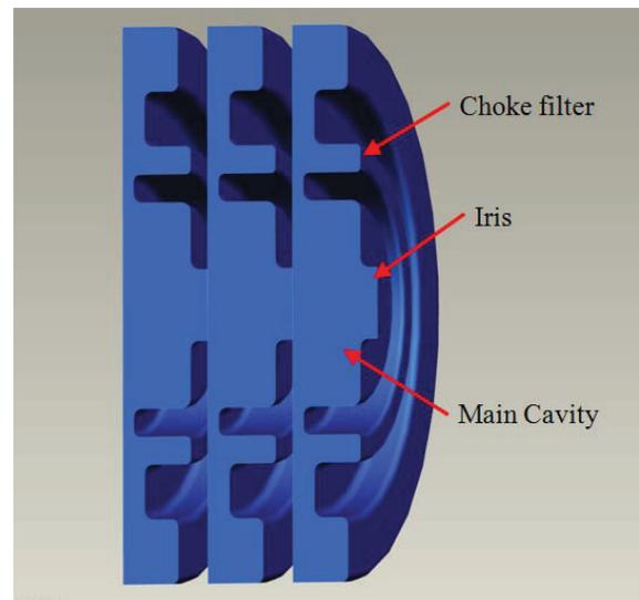
Figure 1: a cross-sectional view of the vacuum volume in the C-band accelerating column.
