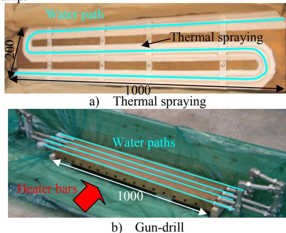
Figure 3: Candidates of cooling device
