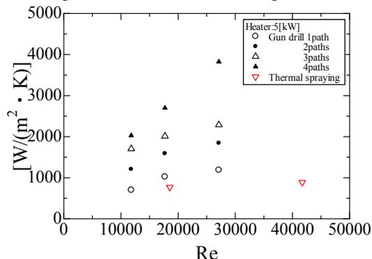
Figure 4: Result of cooling test, x-axis: Reynolds number [-], y-axis: heat transfer coefficient[W/m²/K].
