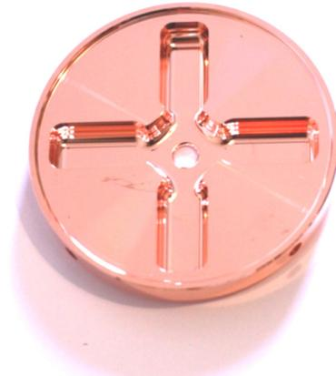
Figure 1: Typical damped cell of TD18 structure.
