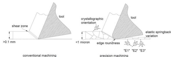
Figure 2: Relative scale comparison of conventional vs. precision cutting processes [4].
