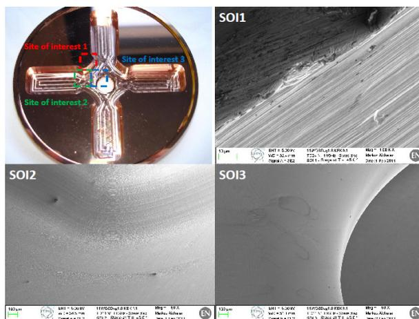
Figure 3: Standard designation of SOI. SOI1: burrs inspection on the top plan; SOI2: radii milling transitions; and SOI3: turning milling transition in the iris.
