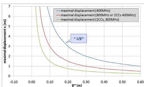
Figure 3: The maximal displacement for  $\sin(\Phi + \frac{\omega z}{c}) = 1$  as a function of the beta function at the IP by a single or two independent 400 MHz or 800 MHz CCs.
