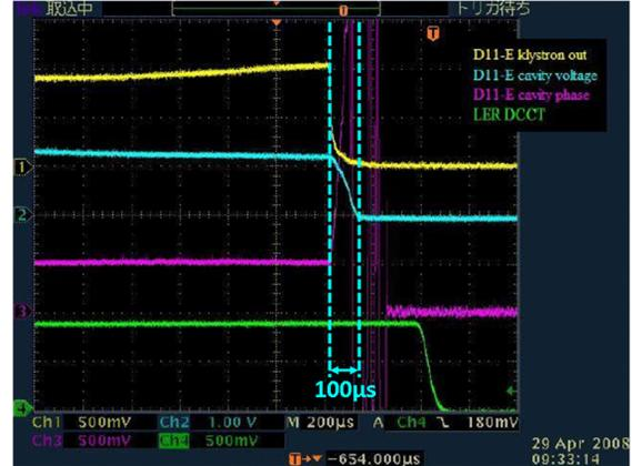
Figure 1: KEK-B CC voltage and phase after a fast failure. The voltage decays completely in  $100 \mu\text{s}$ . Large oscillations of the cavity phase are observed. (courtesy of K. Nakanishi et al. [4])
