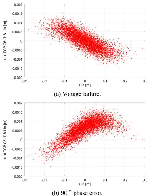
Figure 2: The bunch shape at the primary collimator TCP.C6L7.B1 after an instantaneous voltage change to  $V_0 = 0$  of the CC downstream of IP5 (a) and after an instantaneous  $90^\circ$  phase shift of the CC upstream of IP5 (b) for beam 1.  $x$  denotes the transverse coordinate,  $z$  the longitudinal coordinate. The trajectories of 10,000 particles are tracked using the LHC upgrade optics and single 400 MHz CCs in the local scheme around IP5.
