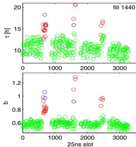
Figure 5: Luminosity evolution dependence on collision schedule: grey for bunch pairs colliding in all IPs; green for collisions in IP1, 5, 8; blue for IP1, 5, 2; red for IP 1, 5.
