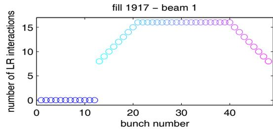
Figure 2: Number of LR encounters per bunch: in blue the 12 non-colliding bunches, in cyan fading to magenta the 36 50 ns spaced bunches.
