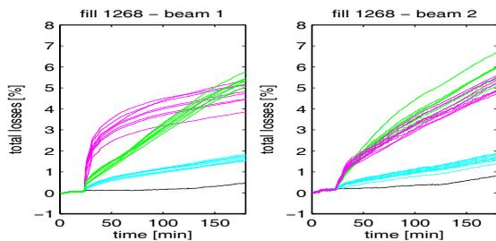
Figure 1: Bunch losses versus time, colour coding to highlight the dependence on the collision schedule: green collisions in IP1, 5 and 8, magenta collisions in IP1, 5 and 2, cyan collisions in IP8 and 2, black non colliding bunch.
