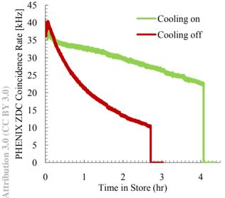
Figure 3: Luminosity lifetime for two similar stores, with and without stochastic cooling.
