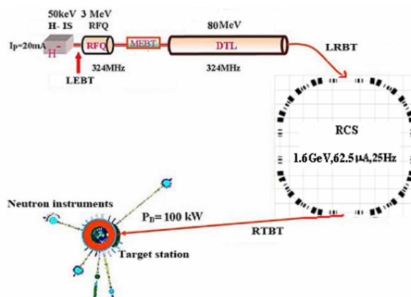
Figure 1: Schematics of the CSNS complex.
