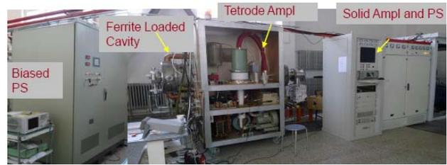
Figure 11: Prototype of RCS RF system.
