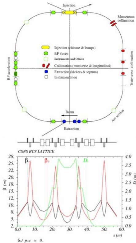
Figure 4: RCS function arrangement (upper) and twiss parameters of one super-period (lower).
