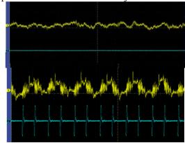
Figure 5: Un-trapped He1+ beam (upper) and barrier bucket trapped He1+ beam (bottom) 10 msec after injection and barrier voltages (sky blue).
