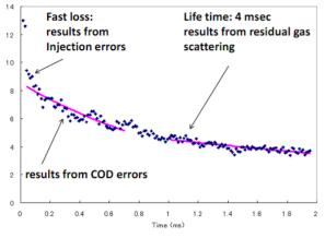
Figure 6: Beam intensity in au after injection.
