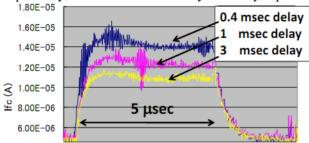
Figure 3: 5  $\mu$ s chopped pulse profiles, which are chopped at different times from the pulse head of a 5 ms ion pulse.
