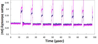
Figure 4: Free circulation of He1+ ion beam; No injection error correction (blue) and with correction (purple).
