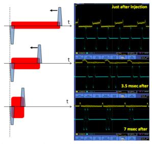
Figure 7: Bunch squeezing experiment (right) and schematic of barrier voltage operation (left).
