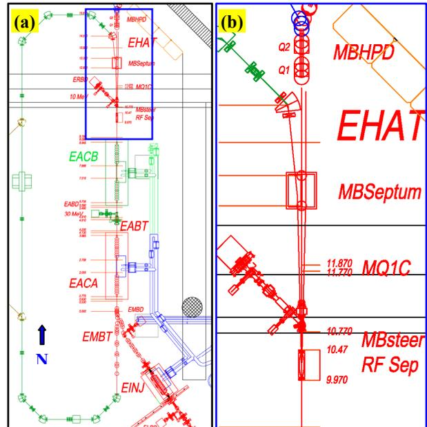
Figure 1: (a). ARIEL Electron Linac and recirculation loop inside E-Hall. (b). RF separation scheme (blue rectangle in (a) magnified).
