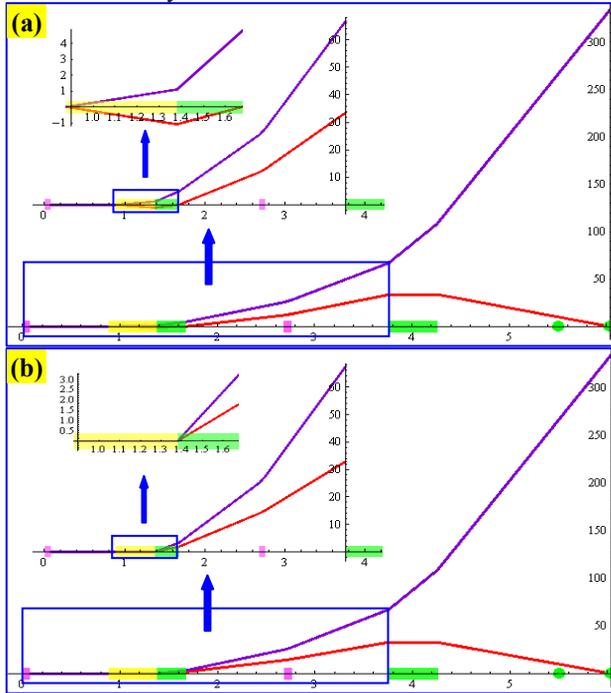
Figure 2: Beam separation geometry in (a) simultaneous ERL-FEL+RIB and (b) 2-pass RLA-RIB modes, showing horizontal offset (mm) vs longitudinal distance (m). Each plot contains 3 layouts of increasing detail, with red/purple line for extracted/recirculated orbit. Coloured elements are, left to right: Magenta: F & D quads; Yellow: RF separator; Green: steering dipole, septum, Locations (circles) of first arc dipole and high power dump dipole.
