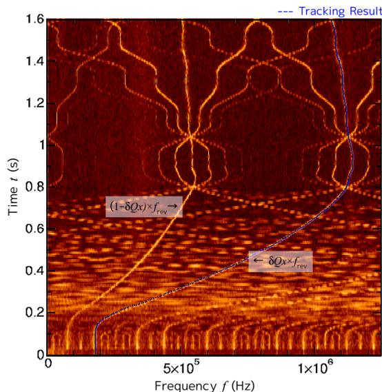
Fig. 2: Temporal evolution of the spectrum distribution for the horizontal oscillation.
