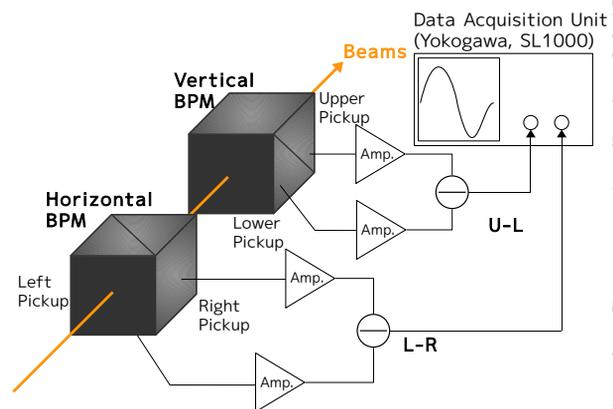
Fig. 1: Schematic diagram of the tune measurements.
