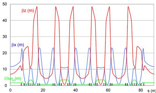
Figure 6: "Low- $\alpha$ " optical functions (one super period).
