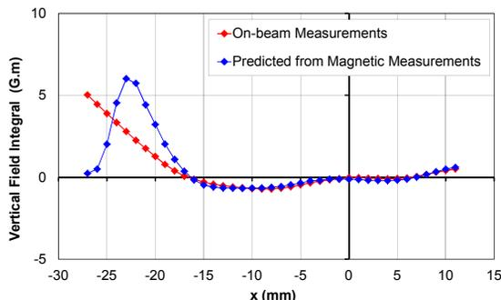
Figure 2: WSV50 vertical field integrals. The x-range is fixed by the maximum allowed orbit bump amplitudes.
