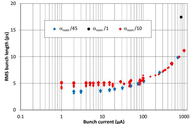
Figure 7: RMS bunch length variation versus bunch current for  $\alpha_{\text{nom}}/10$  and  $\alpha_{\text{nom}}/45$  (RF voltage = 4 MV).
