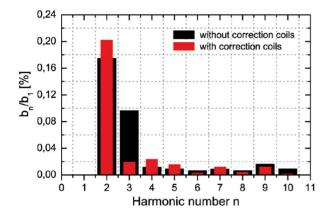
Figure 3: The integrated field harmonics  $b_n$  of the ESR dipole magnet normalized to the main dipole field. The field was analyzed at the reference radius of 5 cm. n = 1,2,3.. corresponds to the dipole, quadrupole, sextupole component etc.
