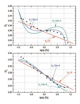
Figure 7: Measured (symbols) and calculated (curves) betatron tunes for the different sextupole harmonic  $b_3$  of the dipole magnets.
