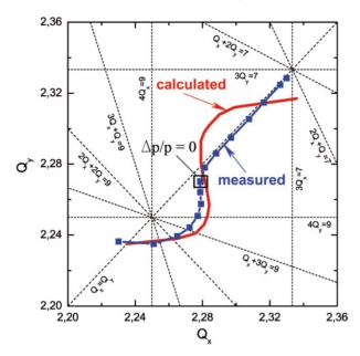
Figure 6: The betatron tunes of the ESR. Each measured point corresponds to a different beam orbit, i.e. value of  $\Delta p/p$ .
