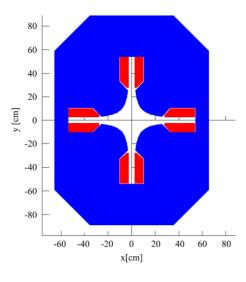
Figure 4: The cross section of the ESR quadrupole magnet.
