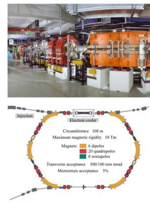
Figure 1: The Experimental Storage Ring at GSI, Darmstadt.
