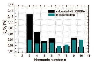
Figure 5: The integrated field harmonics  $b_n$  of the ESR quadrupole magnet normalized to the main quadrupole field. The field was analyzed at the reference radius of 12 cm.
