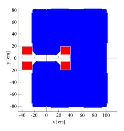
Figure 2: The cross section of the ESR dipole magnet.
