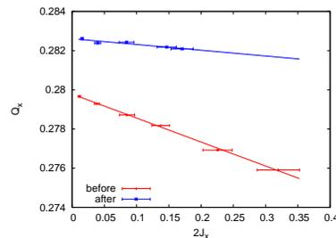
Figure 2: Amplitude detuning of  $Q_x$  for horizontal kicks before (red) and after (blue) correction of the NL-chromaticity.
