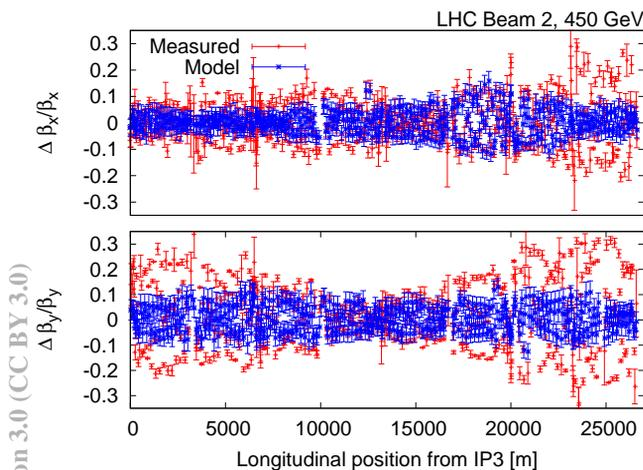
Figure 3: Modeled  $\beta$ -beating together with measurements from the 19<sup>th</sup> of August 2010 for Beam 2 at 450 GeV.
