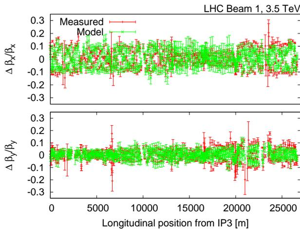
Figure 2: Modeled  $\beta$ -beating together with measurements from the 4<sup>th</sup> of September 2010 for Beam 1 at 3.5 TeV.
