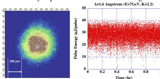
Figure 1: The observed profile of the SASE laser signal at 10keV (left) and the laser intensity stability (~18% fluctuation) during one-hour operation (right).
