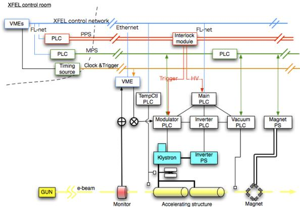
Figure 2: A schematic view of the SACLA control system.
