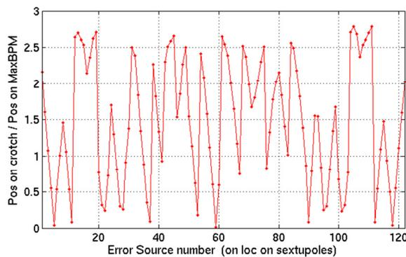
Figure 3: Ratio in the vertical plane between the maximum vertical deviation of the photon beam at the Tomography crotch and the greatest position read by the 122 BPMs. The ratio is computed for each corrector (corrector number is shown on the horizontal axis of the graph). There are only 56 power supplies actually implemented among 122 vertical correctors located in the sextupoles, but all 122 cases are represented here.
