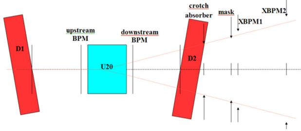
Figure 1: Top view of a short straight section hard X-ray Frontend. The “vertical” scale in the drawing which actually represents the machine horizontal plane is exaggerated in order to clearly see the angular apertures.
