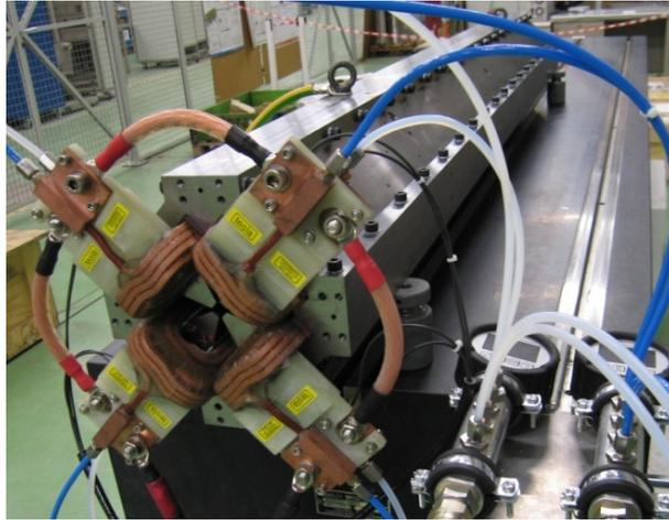
Figure 2: The assembled type4 MBQ magnet.
