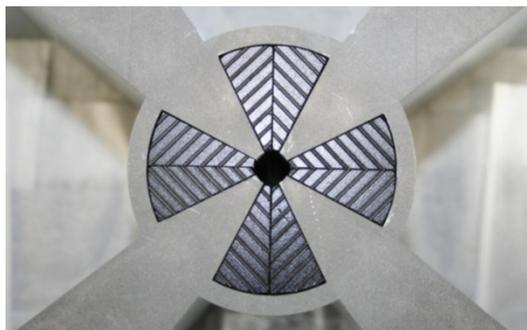
Figure 5: Detail of the QD0 central part assembly.
