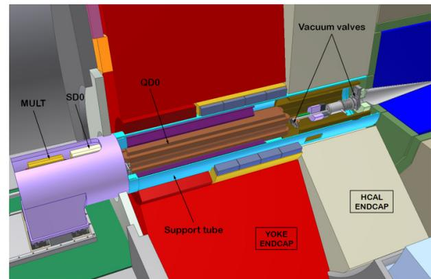
Figure 3: view of MDI with the QD0 inside the detector.
